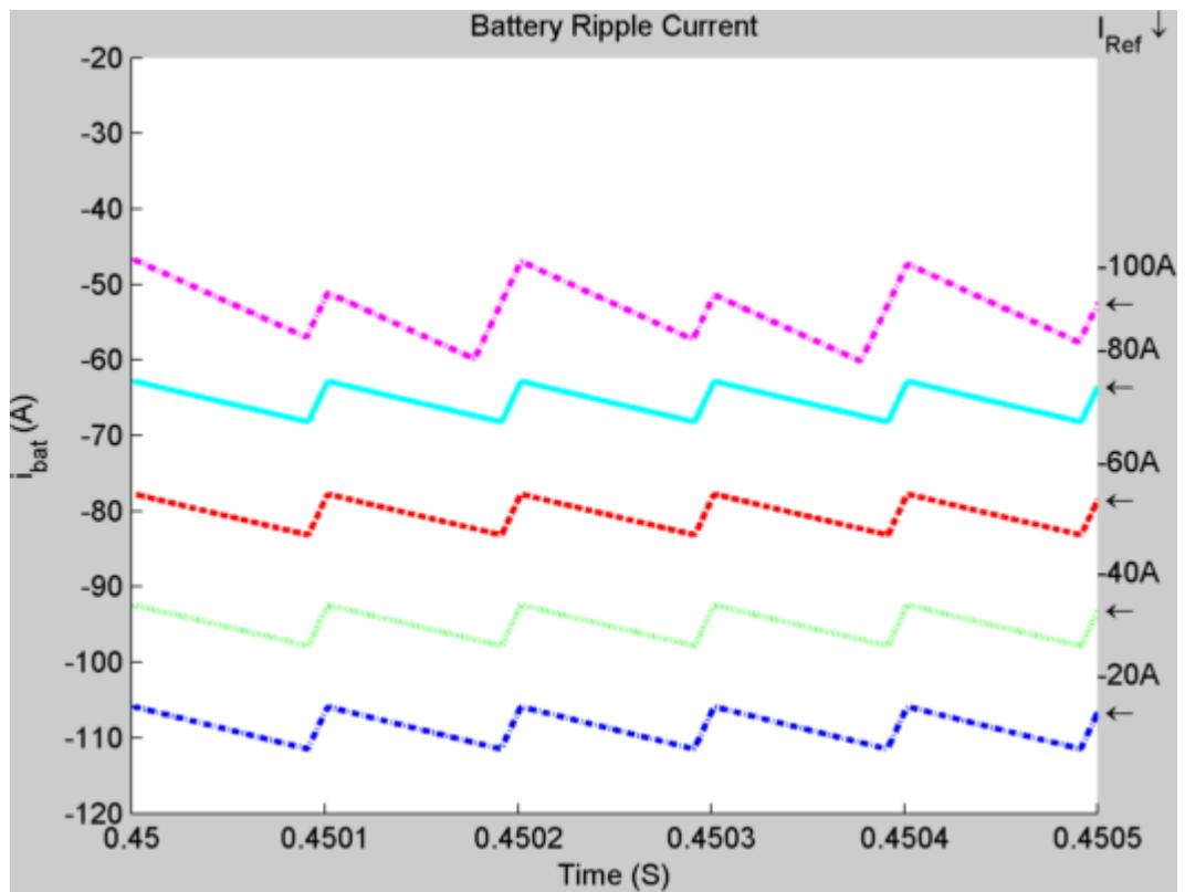
Figure 3.22: Parallel converters - Battery ripple current for varying
