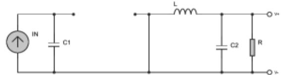
Appendix Figure 4.3: Bus Connected Buck Converter - OFF
