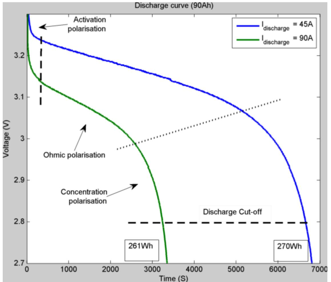
Figure 2.2: Discharge curve for different discharge rates
