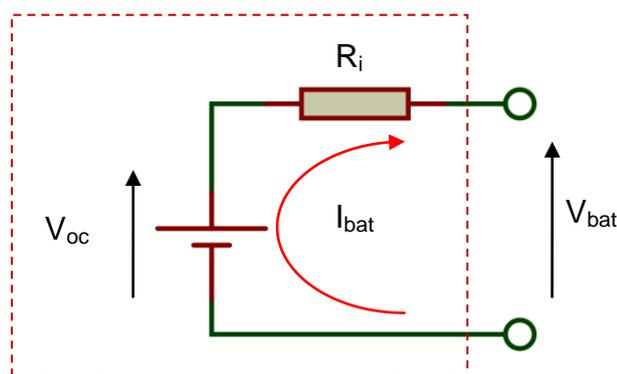
Figure 2.5: Battery as a non-ideal voltage source
