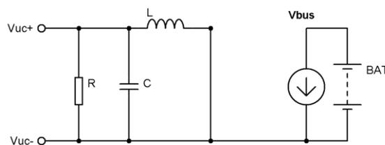
**Figure 3.8: Battery + UC Module – Buck Off**
