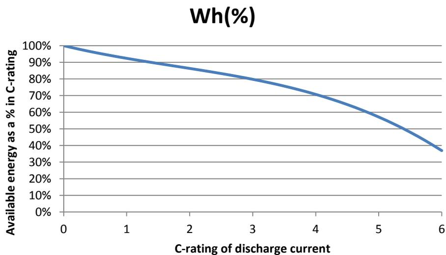
**Figure 3.31: Battery Energy efficiency based on C-rating**
