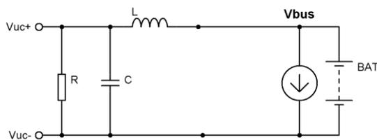
**Figure 3.7: Battery + UC Module – Buck On**
