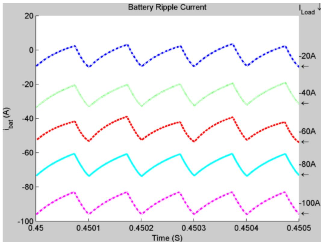
Figure 3.16: Battery ripple (buck-buck) – constant UC module support
