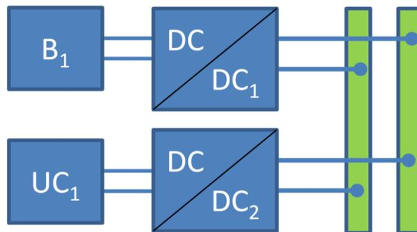
**Figure 2.21: Bi-directional Converter topology**
