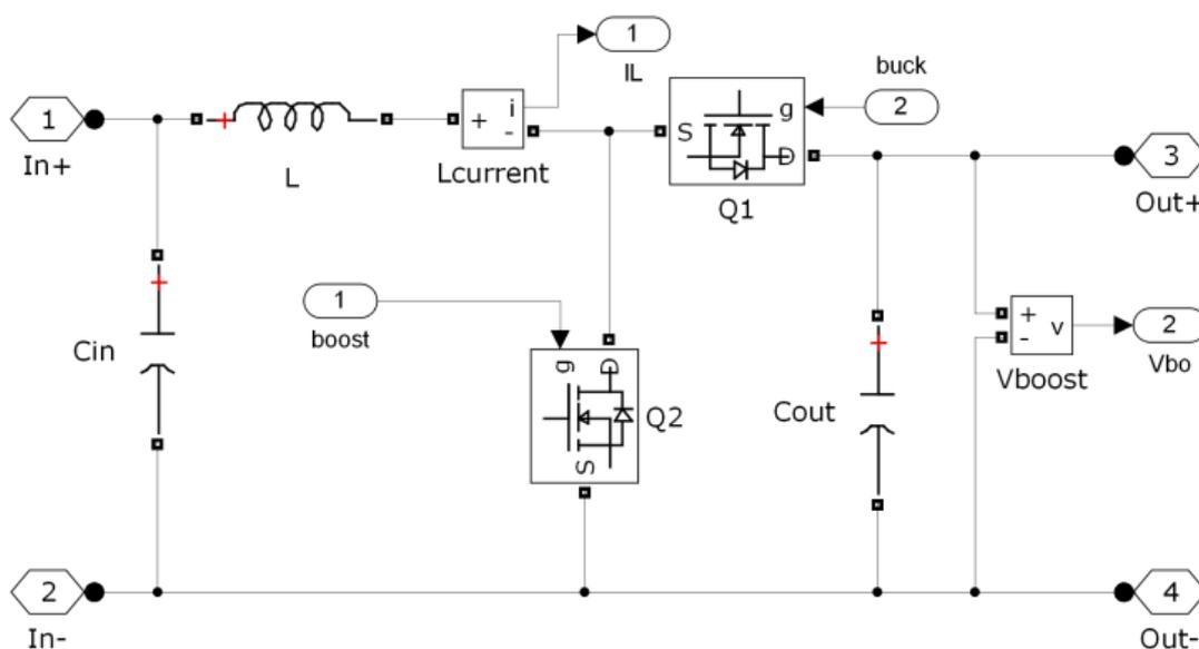
Figure 3.40: Bi-directional DC-DC Converter as modelled in SPS
