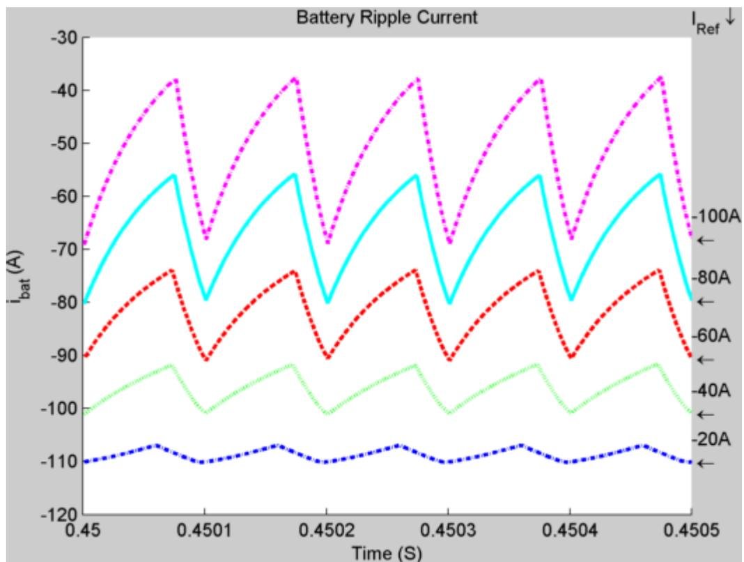
**Figure 3.17: Battery ripple (buck-buck) – constant load demand**
