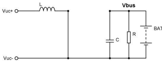
**Figure 3.5: Battery + UC Module – Boost On**
