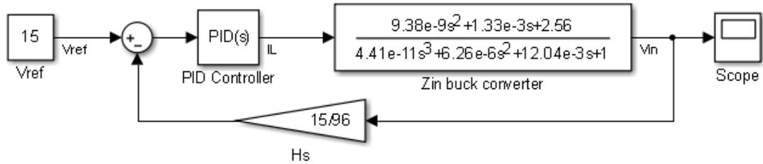
Figure 2.15: establishing control parameters for buck converter
