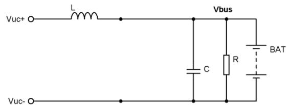
**Figure 3.6: Battery + UC Module – Boost Off**
