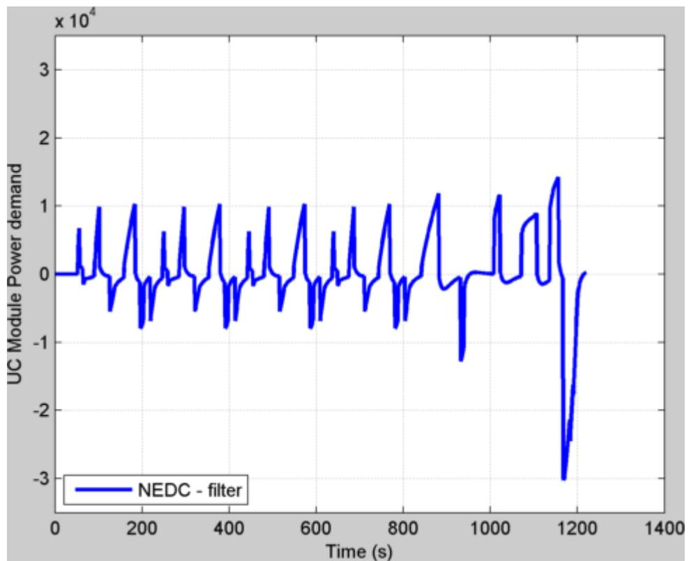
Figure 5.9: Expected UC Module power demand - NEDC
