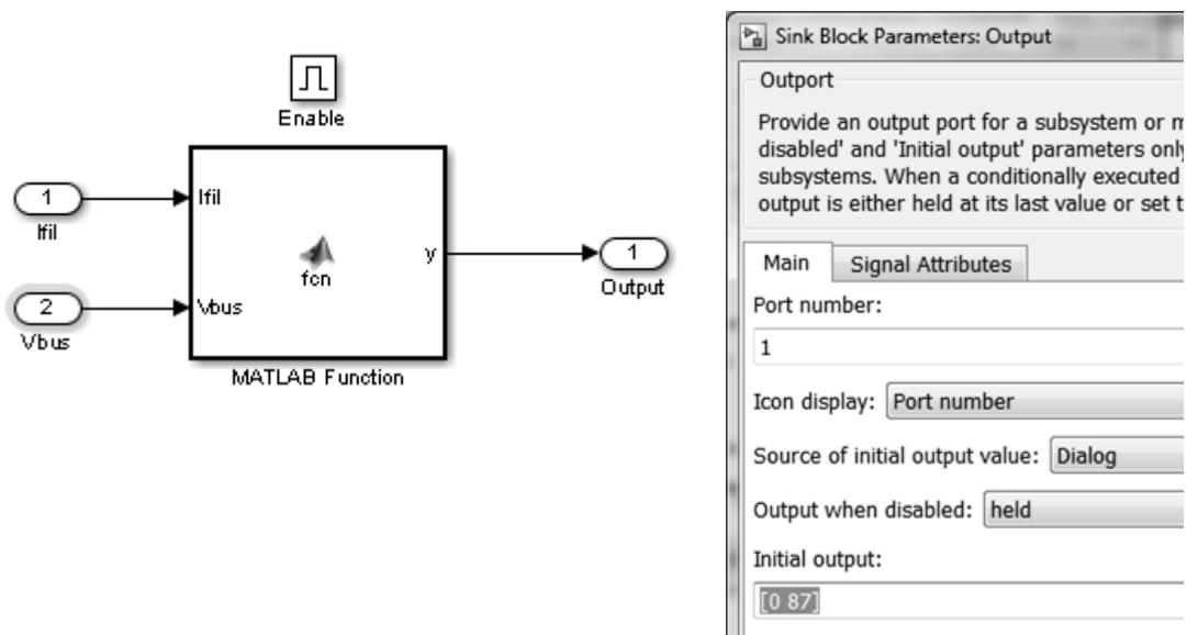
**Appendix Figure 6.1: Enabled Subsystem and output port parameters**
