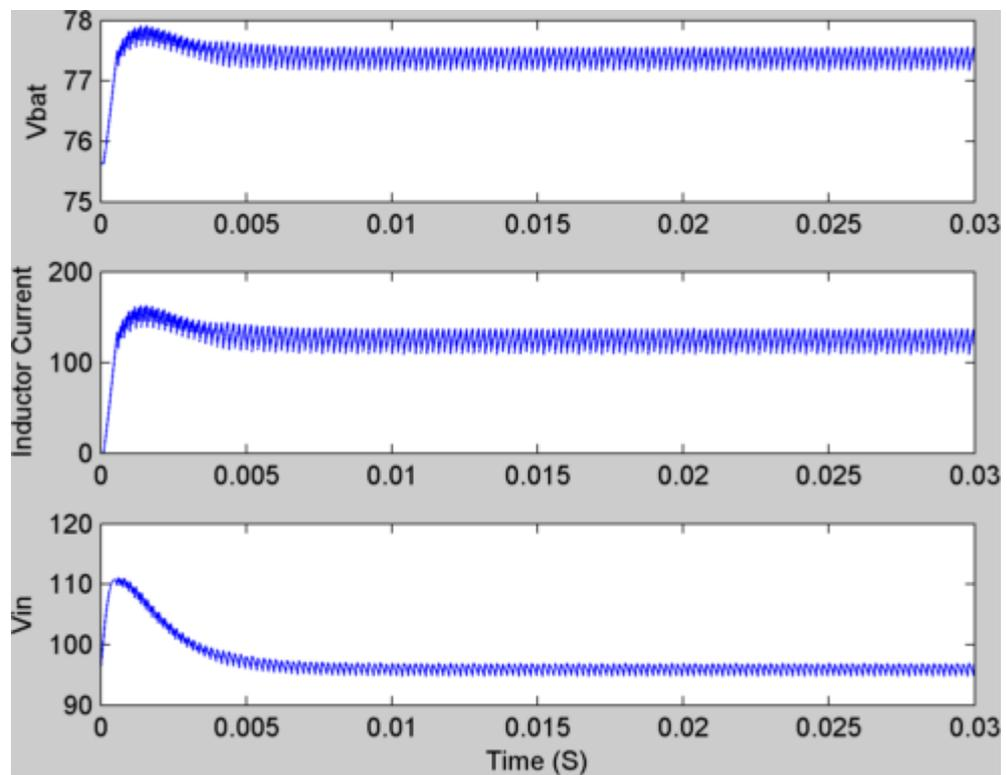
Figure 2.14: Simulation output controlled reference current
