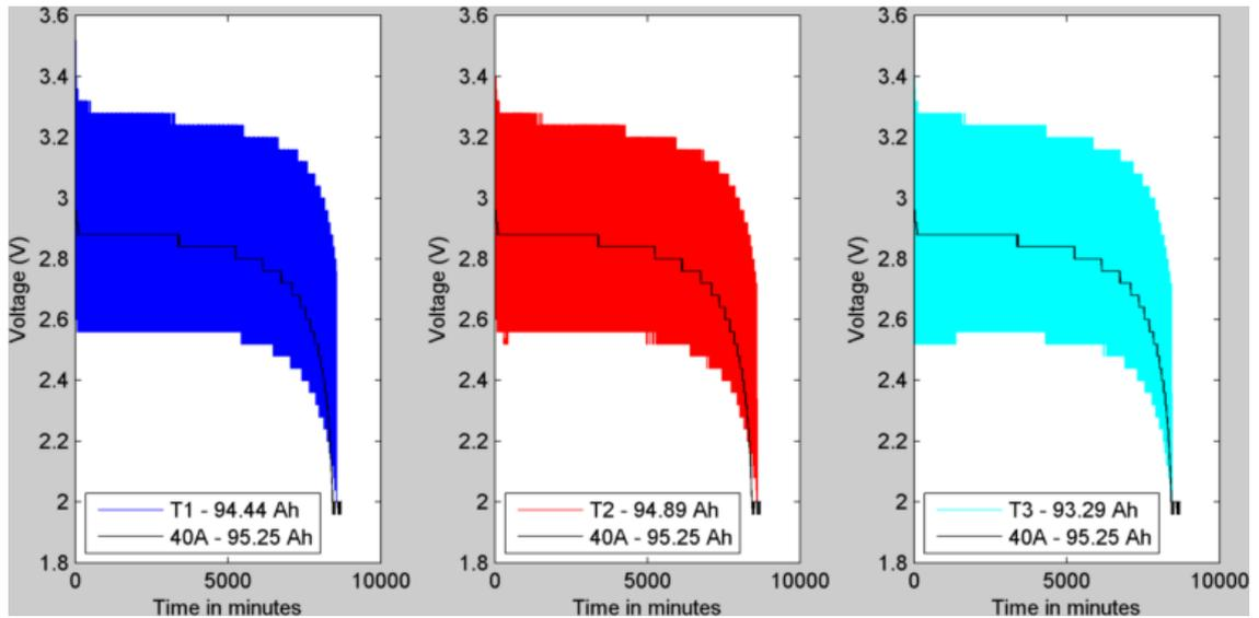
**Figure 3.32: Different pulse test and the resulting capacity**
