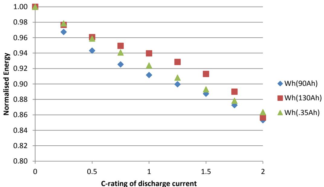
Figure 3.30: Battery test data normalised to C-rating
