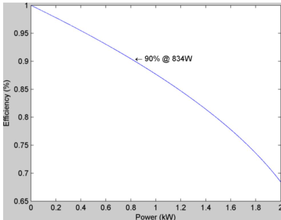
Figure 2.16: UC Cell Power versus Efficiency graph
