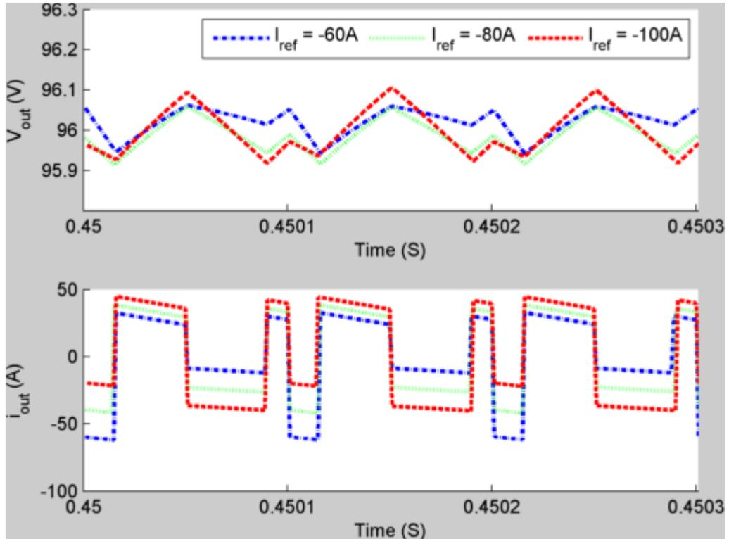
Figure 3.24: Parallel Topology - Bus Capacitor (with timing offset)
