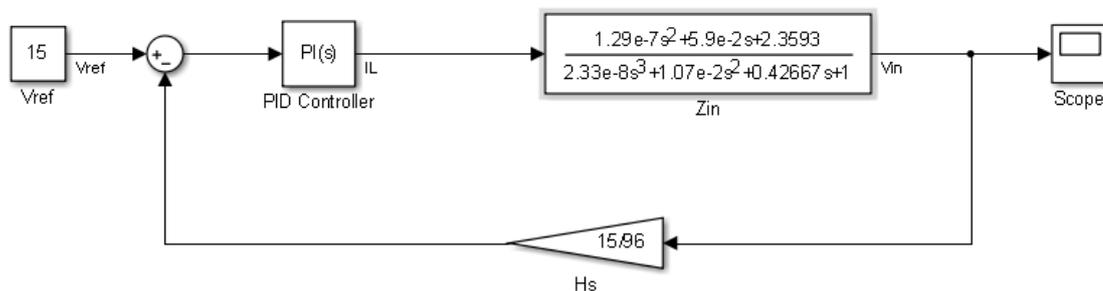
**Appendix Figure 4.5: Buck converter control from Bus voltage**
