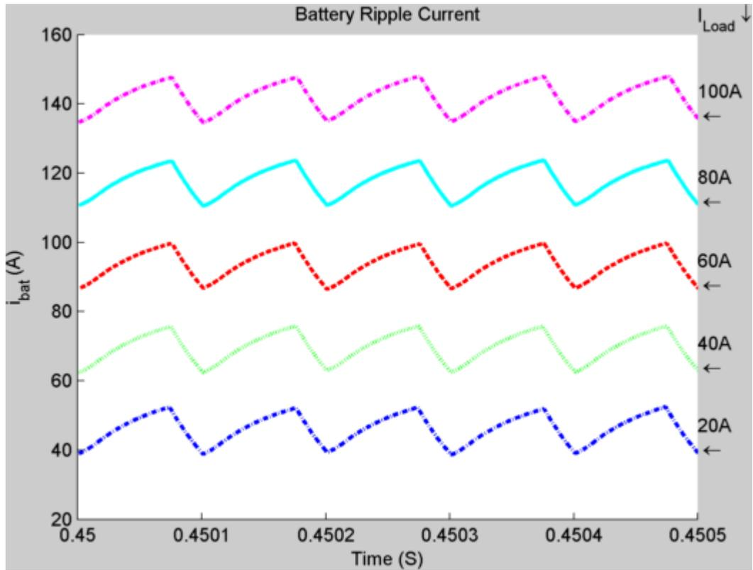
Figure 3.14: Cascaded converters - Battery ripple current for varying Load – Buck Mode
